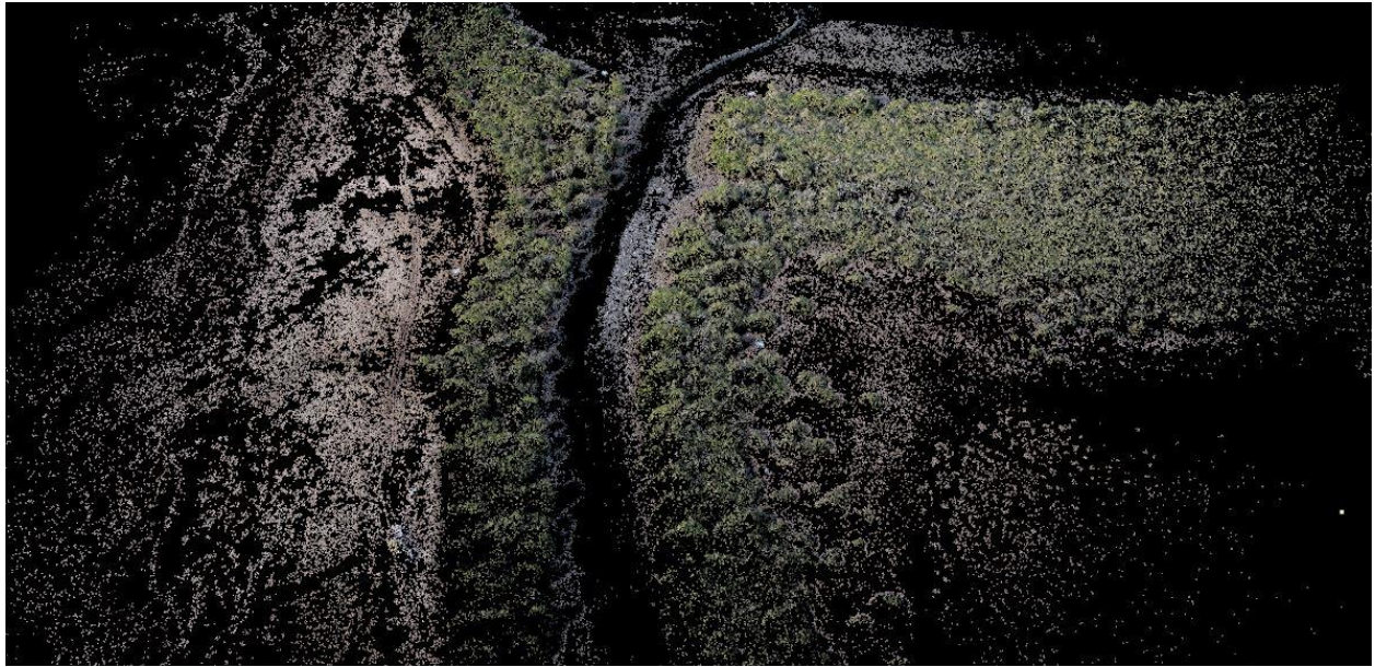
Figure 13. Rough 3D model created through the Initial Processing step. Brighter areas in the center of the image have a higher point density and show location with a higher image overlap.
