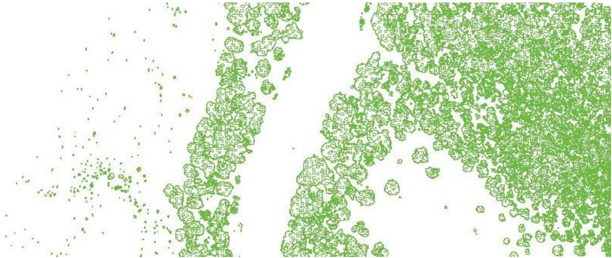
Figure 25. Polygon shapefile of mangrove tree features derived from the ISO classification output after a reclassification of the raster dataset. To clean the data, the area of each feature is calculated and small polygons that are non-tree features such as shrubs are selected and deleted in the editor menu.
