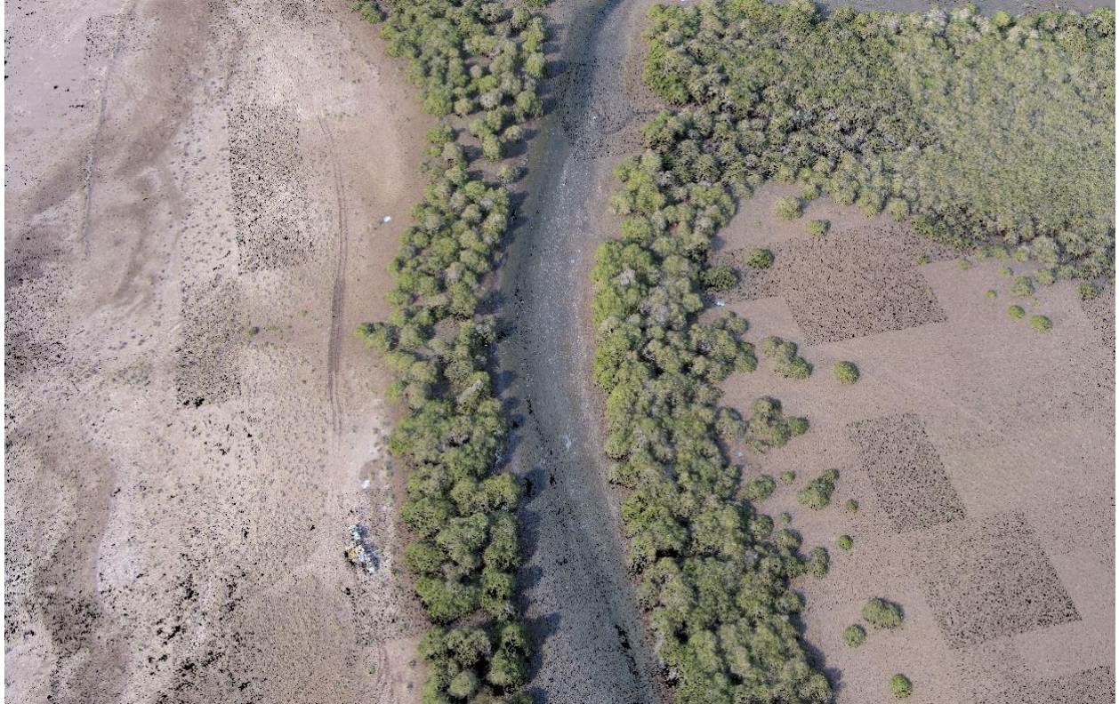
Figure 18. Densified point cloud output from the Point Cloud Mesh tool. Dark areas show lower point density because of low image overlap in that section of our study area.
