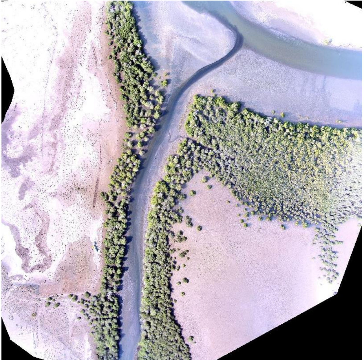
Figure 19. 5cm resolution 4-bands (red, green, blue, and grayscale) orthomosaic image output created from the drone images in Pix4D.
