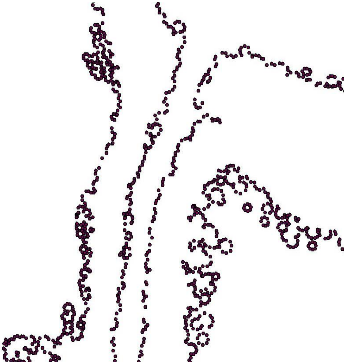
Figure 28. Points created around the mangrove tree features from the tree polygon shapefile. Using the Zonal Statistics tool, we assign elevation values from the DSM to each point.
