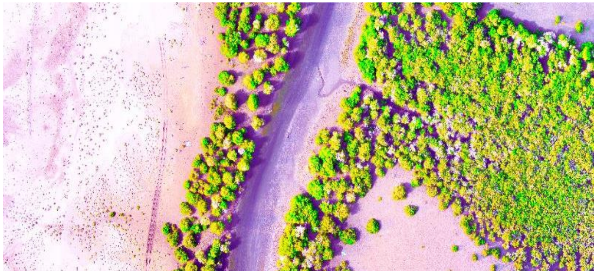
Figure 23. Modified orthomosaic image of the study area to enhance mangrove trees in the image by increasing brightness and saturation values.
