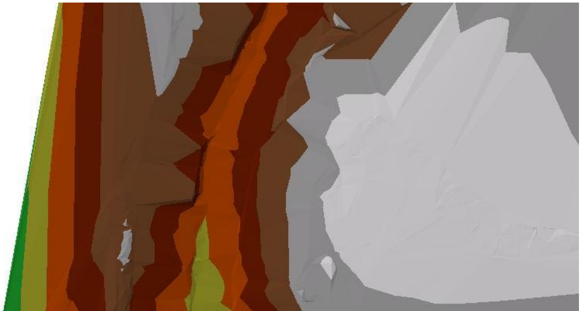
Figure 29. TIN output created using the Create Tin tool in ArcGIS that extrapolates the elevation values from the points created in figure 18 across space.
